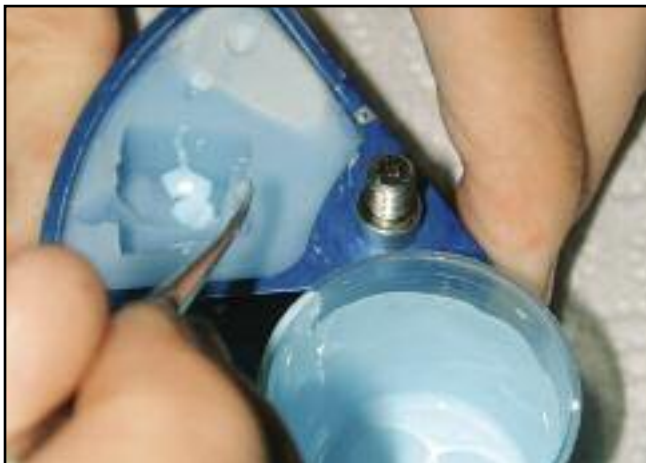
Fig 7 Polyurethane resin was poured into the silicone mold.
