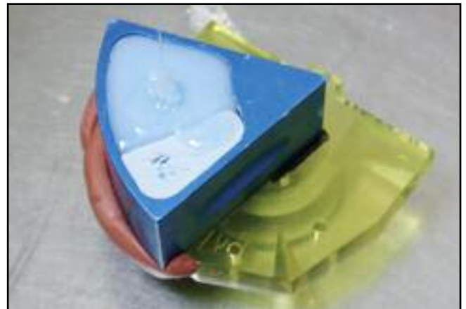
Fig 6 The addition reaction silicon was poured into the flask.
